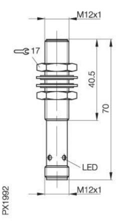
Inductive Sensors BES 516-329-S 4-C M12x1 x 70 normally-open Sn=2mm shielded
